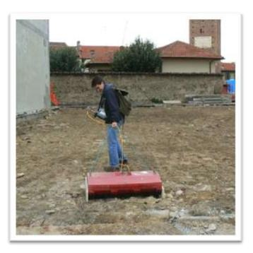
depth of penetration, but have poorer spatial resolution; higher frequency antennas provide less penetration but higher resolution.
