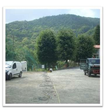
wavelengths are sensitive to the physical properties of near-surface layers. This noninvasive method is used to produce a Vs profile through spectral analysis of surface waves.
