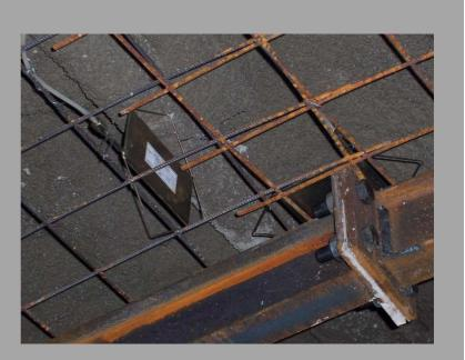
The cell consists of a rectangular flat jack formed from two plates of steel welded around the periphery. The narrow gap between the plates is filled with de-aired oil. The cell is connected to a pressure transducer by a short hydraulic tube and equipped with a re-pressurizing valve. Cells can be embedded in concrete and they are suitable for monitoring by NATM method.
